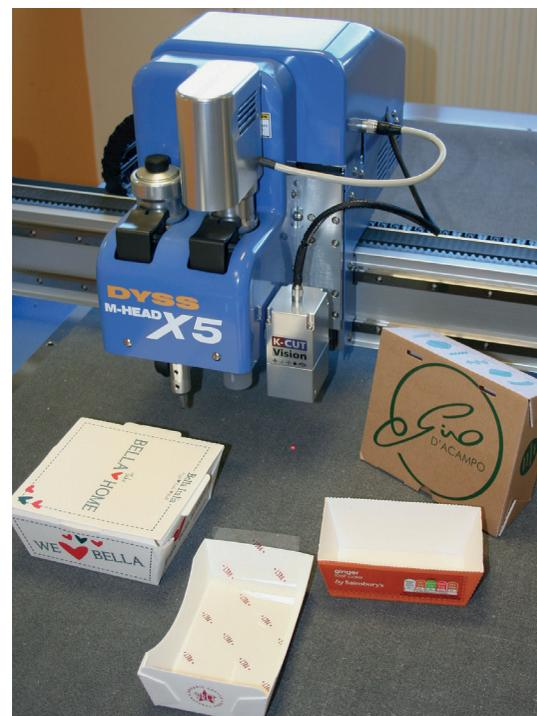
“HUHTAMAKI TESTED THE VARIOUS CUTTING MACHINE VENDORS WITH LIGHTWEIGHT GLASSINE PAPERS THAT IT FREQUENTLY MANUFACTURES TO PROTECT CHOCOLATES IN CONFECTIONARY BOXES FOR HIGH STREET RETAILERS. WITH A HIGH FREQUENCY OSCILLATING KNIFE AND IN PARTICULAR THE CUTTING KNIFE GEOMETRIES CAPABLE OF DELIVERING HIGH QUALITY EDGES WITHOUT TEARING THE DIFFICULT TO PROCESS PAPER, EVEN AT HIGH SPEEDS, AG/CAD WAS SUCCESSFUL WITH THIS TRIAL”
